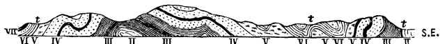
Section from the Great North to the Little North Mountain, through Bore Springs, Va.; t, t, positions of thermal springs.
